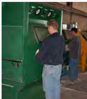
BLAST CABINETS FOR SMALL & DELICATE ITEMS
